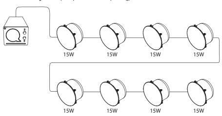
Total Amplifier Load 120W (not including other parasitic loading, always allow amplifier headroom)
